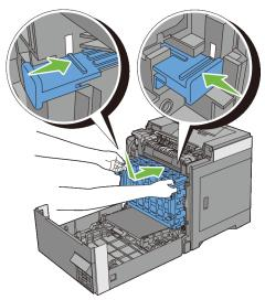
6 Turn the four PHD lock levers 90-degrees clockwise to lock the PHD unit.
